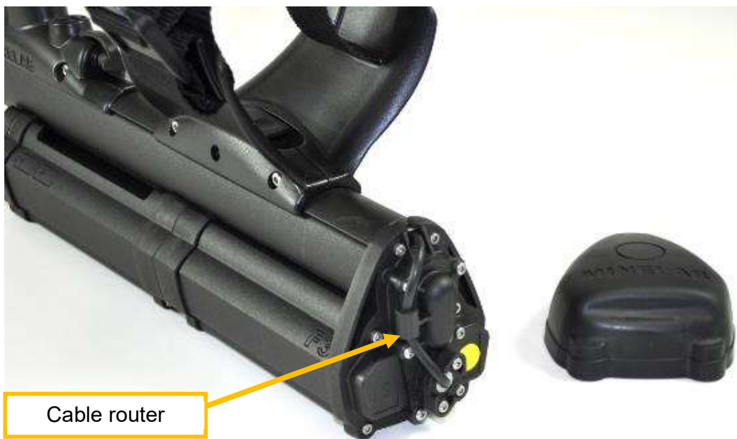
Figure 18: Wiring Loom under cable router.
