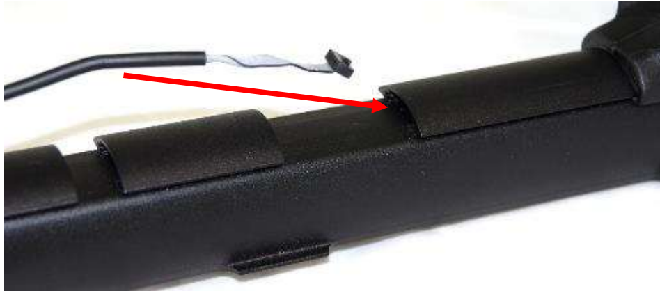
Figure 52: Inserting wiring loom.
